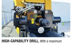
torque of 110 kNm, the D120E delivers the hole-making capability comparable to a larger maxi rig. The direct, electric drive results in reactiveness, controllability and scalability of the rig for highly efficient operations.
