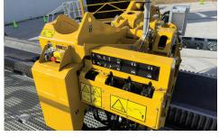
**EXTENDED DRILL PIPE RANGE.** The powerful vise travels along the full length of the rack. With 220 kNm of breakout torque and 110 kNm of makeup torque, the vise makes it possible to use drill pipes up to 7,625-in outer diameter. Thanks to a large passthrough opening, the vise makes it possible to handle tooling and steel casing with an outer diameter up to 406 mm (16-in).
