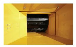
FEED ROLLER. A large letterbox infeed opening at 44 cm x 30 cm (17 .5 in x 12 in) helps boost productivity by reducing the need to trim material before feeding it into the chipper.
