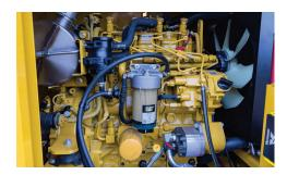
POWERFUL PERFORMANCE. The 74 hp (55 kW) Stage V compliant Caterpillar diesel engine allows you not only to comply with Stage V emissions requirements, but also gives you the engine power to meet your jobsite needs.
