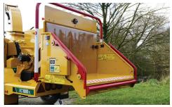
**SMARTFEED.** The SmartFeed system monitors engine rpm and automatically stops and reverses the feed rollers to maximize productivity. This system also senses feed roller jams and manipulates the material automatically to reduce the need for manual control bar use.
