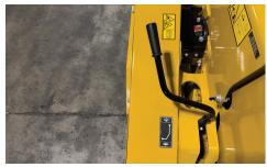
**CLUTCHLESS PTO SYSTEM.** A clutchless PTO system allows the cutter to be engaged without using a traditional slip clutch or idler pulley and without sliding the engine. The system is convenient to maintain — once under the shield, belt changes are efficiently accomplished without the use of tools.
