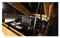
**POWER FOR THE JOB.** The XTS1250i2 is powered by a 127 hp (95 kW) Deutz TCD3.6L diesel engine which offers efficient power for working in difficult ground conditions.
