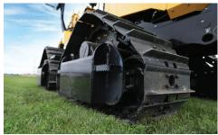
**STEEL QUAD TRACK SYSTEM.** Four independent steel tracks can offer enhanced floatation and traction with four-wheel and crab steering options.
