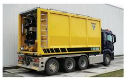
**COMPACT SIZE/EFFICIENT TRANSPORT.** Based on 20 ft ISO container dimensions, transport dimensions are minimized. The shaker module ships inside the tank. During setup, the module can be lifted out and installed by turning it one-quarter of a turn.
