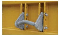
**HOOK LIFT SYSTEM.** The MR1000 reclaimer is available with a height-adjustable hook lift system with low- or high-profile rollers to fit local transport requirements.
