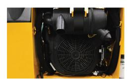
25 HP (18.6 KW) EFI ENGINE. Starts well during cold weather, makes choke cables obsolete and offers improved fuel economy over comparable carbureted gas engines.
