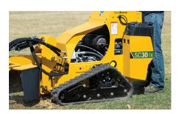
HYDRAULICALLY DRIVEN CUTTER WHEEL AND GROUND DRIVE. The elimination of belts or chain drives reduces service and maintenance.
