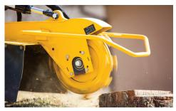
PATENTED YELLOW JACKET™ CUTTER **SYSTEM.** The Vermeer-exclusive Yellow Jacket cutter system is designed to provide faster, easier serviceability, as well as extended pocket and tooth life.
