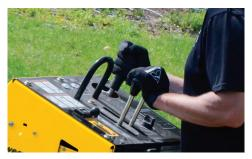
**OPERATOR PRESENCE SYSTEM.** Control handle for the boom swing and boom raise/lower is equipped with operator presence capacitance-sensing handle. This system is intended to help protect the operator.
