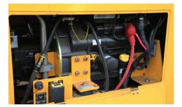
**ENGINE.** The TR6400 features a Deutz 3.6L Tier 4F (Stage IV), 100 hp (75 kW) engine. The engine is mounted on a pivoting frame that swings out 30 degrees for access to fuel filters and hydraulic reservoir for maintenance and service.
