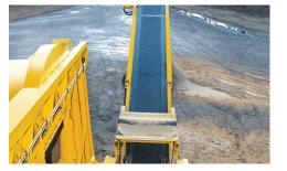
**HIGH PRODUCTION.** Designed to handle more production with less clogging, the 36" (91.4 cm) wide continuous undermill conveyor system offers optimum speed and capacity.
