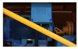
**ELECTRIC MOTORS.** Equipped with a 500 hp (373 kW) WEG totally enclosed fan-cooled electric motor to power the mill. A separate 60 hp (44.7 kW) electric motor powers the pump for the hydraulic circuits, while a 2 hp (1.5 kW) electric motor powers the fan to cool the hydraulic system.
