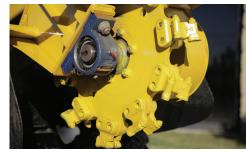
**OPTIMIZED WHEEL.** The SC382 stump cutter wheel has an optimized profile and tooth pattern to help with productivity and chip flow of recirculating material.
