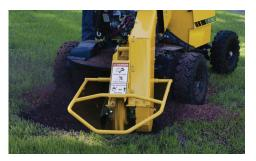
AUTOSWEEP® CONTROL SYSTEM. The optional AutoSweep control system monitors engine speed and automatically adjusts cutter wheel sweep rate, and is designed to reduce engine, drivetrain and structural stress.
