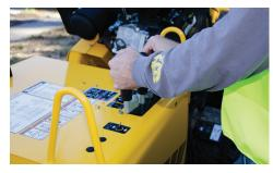
**OPERATOR PRESENCE SYSTEM.** Control handles for boom swing, boom raise/lower and machine propel are equipped with an operator presence feature. This user-friendly operator presence system is intended to enhance operator safety.
