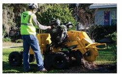
**POWERFUL STUMP REMOVAL.** A 35 hp (26 kW) Vanguard engine offers low vibration, low emissions, smooth easy starting, extended starter life and an instant return to maximum power. Also offers a limited 3-year warranty from Vanguard.
