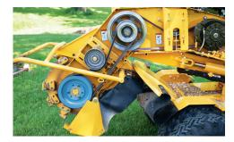
**CONVENIENT BELT SERVICING.** Belts on the SC362 are serviceable from one side of the machine with cutter drive belts being adjustable with movable idlers. Additionally, each belt set may be adjusted independently, without affecting adjustment of other belts.
