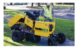
**2-SPEED GROUND DRIVE.** The operator may choose to operate in a high-range ground speed setting of 67 - 133 fpm (20.4 - 40.5 m/min) to quickly move the machine or choose a slower speed when near the stump by utilizing a low-range setting of 0 - 66 fpm (0 - 20.1 m/min).
