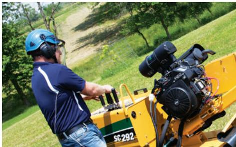
**TWO-SPEED GROUND DRIVE.** The operator may choose a high-range or low-range ground speed setting of 0 – 133 fpm (0 – 40.5 m/min) to quickly move the machine or choose a slower speed when near the stump by utilizing a low-range setting of 0 – 66 fpm (0 – 20.1 m/min).
