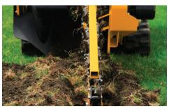
**OUTBOARD BEARING SUPPORT:** This feature provides protection for the headshaft when trenching in difficult conditions, helping to lower the overall cost of operation.
