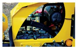
**OPERATORS, START YOUR ENGINE.** The 25 hp (19 kW) Kohler electronic fuel-injected (EFI) gasoline engine offers improved fuel economy reducing greenhouse gas by an average of 25 percent — as compared to conventional carbureted engines. And, best of all, makes choke cables obsolete. Simply put, it's time to start your trencher like you would your car.
