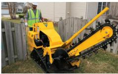
SLENDER PROFILE DESIGN. A 34.5" (87.6 cm) width helps the unit fit through tight areas and narrow gates.
