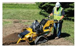
**ENHANCED VZ STEERING.** Operators can steer the machine using only the handlebars — rather than traditional methods using levers or steering wheels. These bars also provide additional leverage when operating on difficult terrain.
