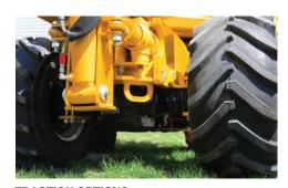
TRACTION OPTIONS. With a variety of different traction options, the PTX40 is well-suited to contractors' differing needs. The 23" (58.4 cm) tire option is best for narrow, congested jobsites, the 26" (66 cm) tire option provides better traction, and the dual tire option accommodates lower ground pressure requirements. Additionally, the PTX40 is available with tracks that are ideal for uneven terrain.
