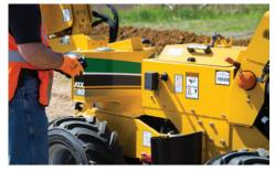
**REMOTE CONTROL.** When plowing or in transport mode, remote control operation offers flexibility in congested areas, providing the operator both fingertip control and smooth machine handling. The remote control functionality provides adjustability for the operator to maintain visibility to the work area and machine operation from a variety of viewpoints. When trenching, the operator controls utilize a tether that connects the machine and remote control.
