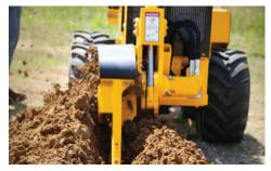
MACHINE VERSATILITY. Utilized for irrigation and utility installations, the versatile PTX40 is a plow/trencher with a dedicated plow depth of up to 24" (61 cm), a trench depth of up to 42" (106.7 cm) and a width of 4-6" (10.2–15.2 cm). The optional bore attachment has a maximum torque of 494 ft-lb (670 Nm).
