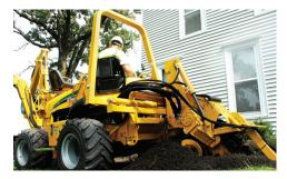
TIRE OPTIONS. The RTX550 is available with standard 31 in (78.7 cm) tires. For even greater flotation, choose the 35 in (88.9 cm) tire option.
