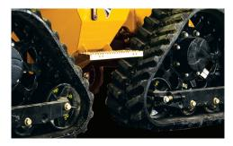
SEE THE DIFFERENCE. When equipped with the innovative quad track system, the RTX550 offers improved flotation, reduced surface damage, increased tractive effort and greater stability. Four-wheel steer and crab steering are functional with the system.
