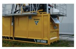
**SMART TRANSPORT, LINEAR JOBSITE.** To minimize transport dimensions, the shaker module ships inside the tank. During setup, thanks to a self-erecting hydraulic system, the module can be lifted out and installed on top of the container ready to work. The unit's in-line architecture, with a blind side wall, makes it ideal for linear jobsites alongside roads.
