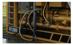
**MIXING PERFORMANCE.** The mixing system is equipped with a powerful vacuum suction system to work efficiently with big bags. A venturi plus a heavy-duty 4 kW, 600-rpm agitator located in the active tank allows for optimum mixing.
