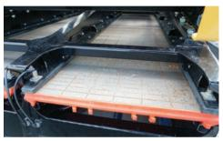
**QUICK-CHANGE SCREENS.** The primary screens are kept in place with an air clamping system, powered by an onboard air compressor. This allows for ease of access and the ability to quickly change screens.
