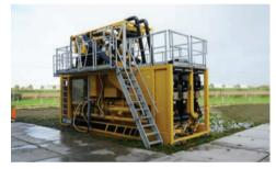
**SMALL FOOTPRINT, BIG PERFORMANCE.** The MR2000 combines both a mixing and reclaiming system, all with a narrow footprint. This compact machine is capable of processing up to 2.000 L/ min of drilling fluid, while transporting just one machine to effectively perform two critical functions on a horizontal directional drilling jobsite.
