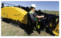
**MAXIMIZE PRODUCTIVITY.** With 24,000 lb (106.8 kN) of thrust/pullback and 3,000 ft-lb (4067.5 Nm) of rotational torque, the D23x30 S3 offers a sizable increase in power over its predecessor, the D20x22 Series II — helping to maximize machine and jobsite productivity.
