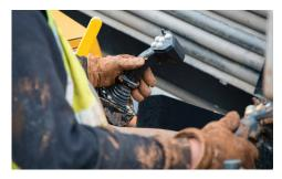
**COMMON CONTROLS.** To assist in operator efficiency and training, the D23x30 S3 features the dual joysticks and common control platform found up and down the Navigator horizontal directional drill lineup. The system design uses less wiring and fewer fuses for greater reliability.
