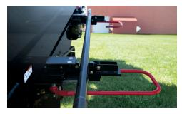
**VARIETY OF ROD OPTIONS.** The D40x55 S3 is available with a range of drill rod options, including a 10' (3 m) length in 2.38" (6 cm) or a 2.63" (6.7 cm) diameter, and a 15' (4.6 m) length in a 2.63" (6.7 cm) diameter. A variety of rod options allows the drill to be configured to the specific needs of the contractor.
